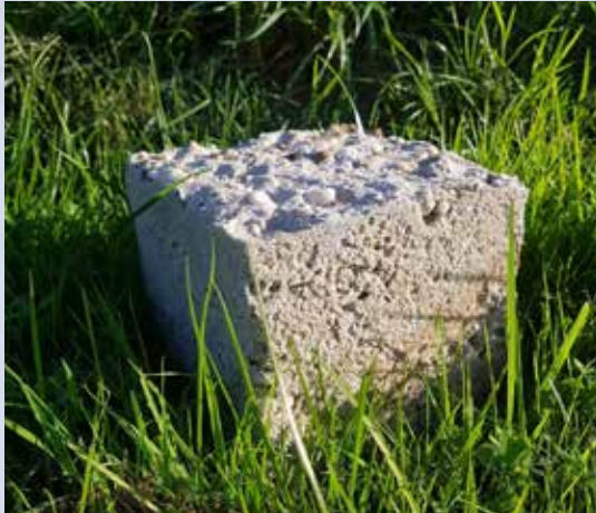
A block of bioconcrete, the production of which extracts CO 2 instead of emissions
